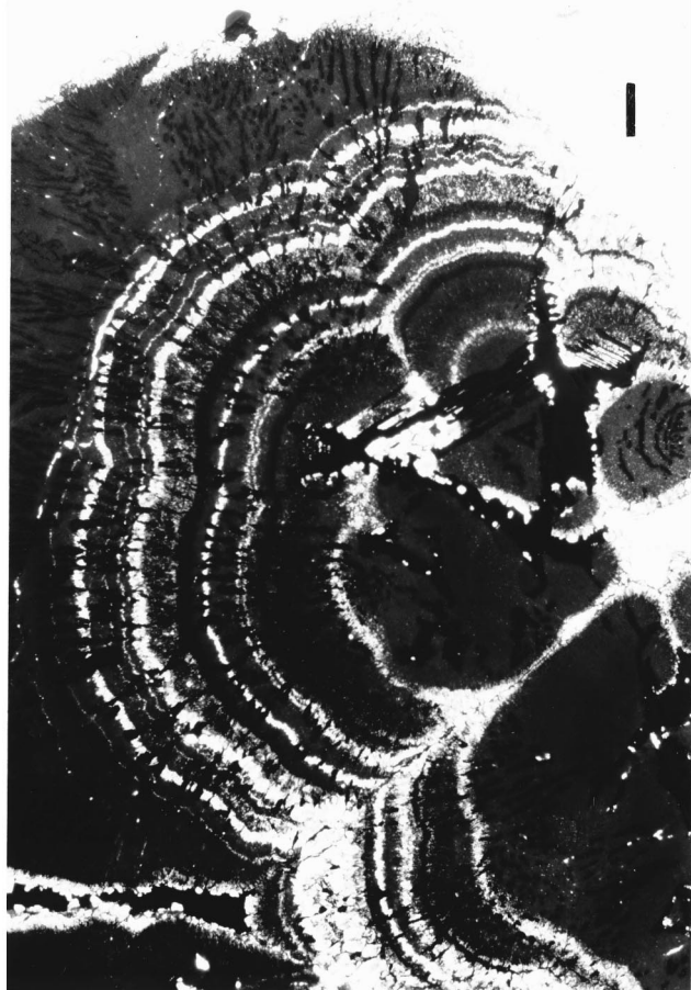
FIG. 1. Microphotograph in transmitted light of a thin section of MVT, sphalerite showing banding, characterized by an alternation of dark and light zones. The concentric bands form crystallite aggregates that emanate from centers of growth. The black filaments are branching galena (PbS) crystals, a mineral often associated with sphalerite. The sample originates from the Polaris mine, Northwest Territories (Canada). The vertical bar in the upper right corner corresponds to 1 mm.
